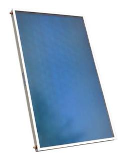
Flat plate collector of 1802 W output (at 1000 W/m² irradiance), designed for onroof portrait installation. A harp absorber with highly selective TiNOx surface is laser welded to the copper pipes. The insulation consists of 40 mm mineral wool. Connections are located on both sides on the top and bottom.
