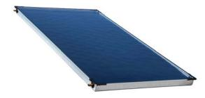
Flat plate solar collector of 1882 W output (at 1000 W/m² irradiance) designed for either portrait or landscape on-roof installation. A harp absorber with highly selective TiNOx surface is laser welded to copper tubing. The insulation consists of 40 mm mineral wool. Connection points are located laterally on the top and bottom.
